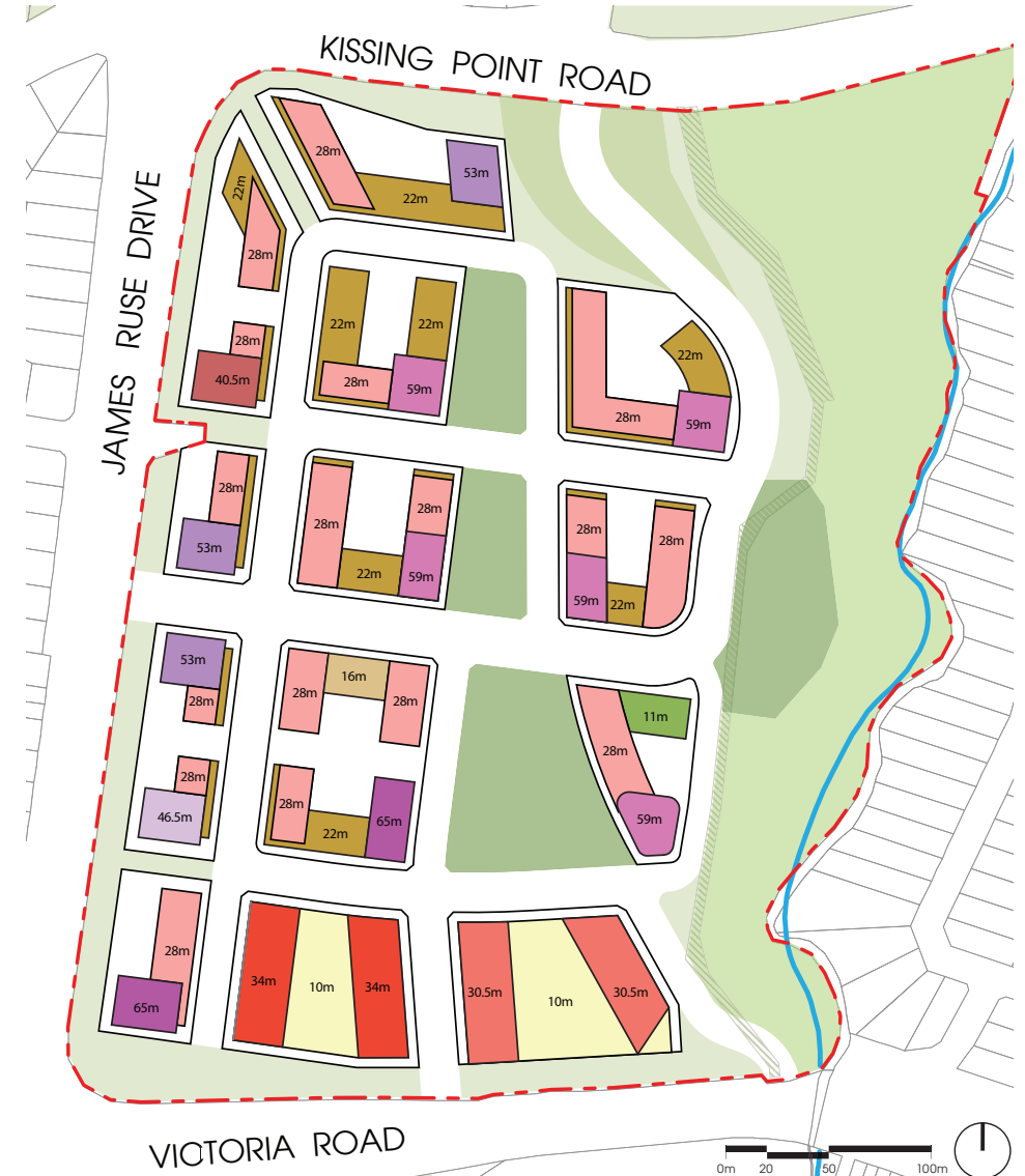
PROPOSED BUILDING ENVELOPES PLAN (HEIGHTS IN METRES ARE ABOVE LOCAL GROUND LEVEL)
